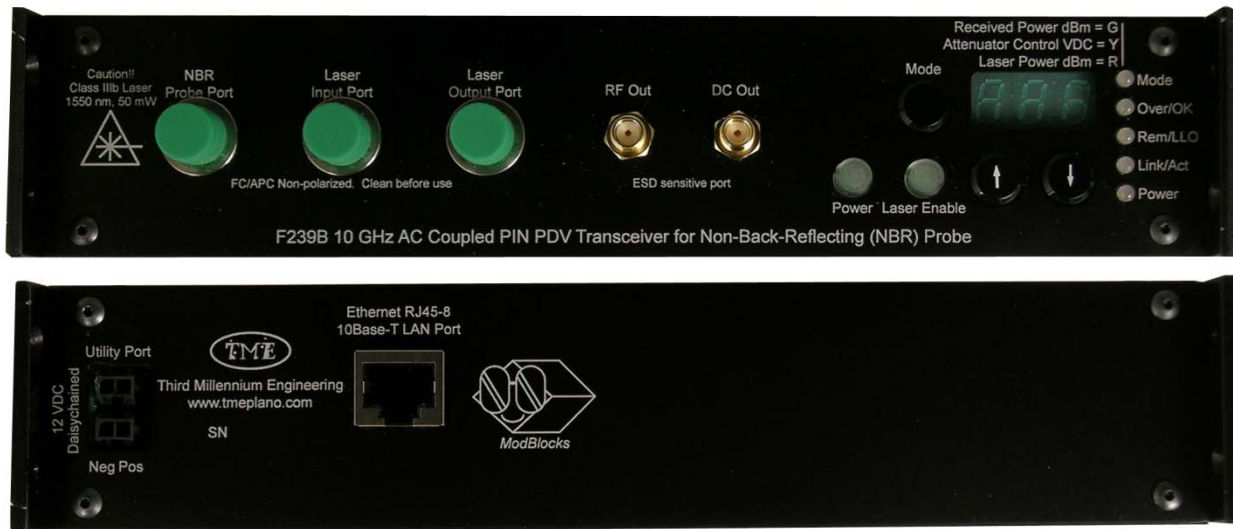
Figure 6. F239B, 1-Channel PDV Transceiver, front and rear panel views
