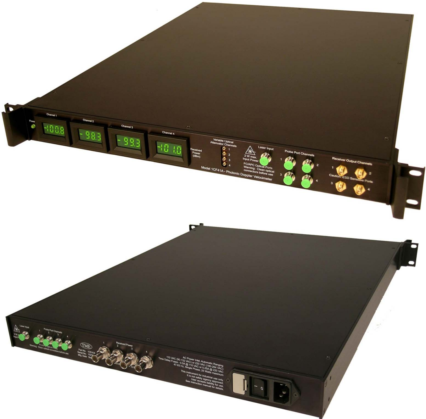
Figure 50. Fiber Optic Doppler Velocimeter, 1CF41A, front and rear views
