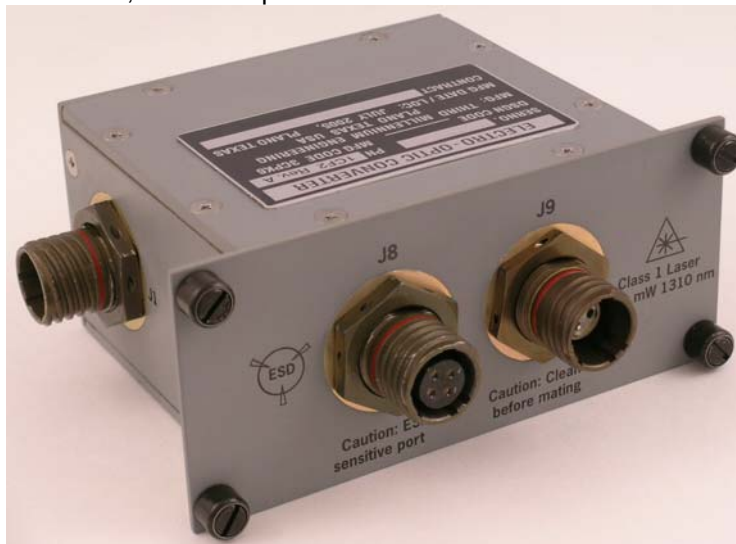
Figure 44. Front View of Ruggedized Fiber Optic Receiver, 1CF2
